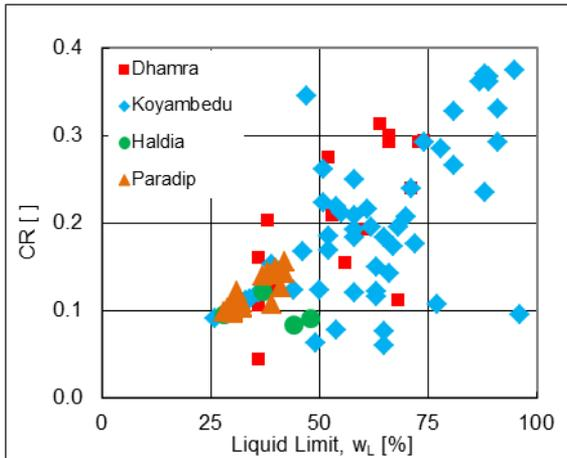
Fig. 4 Plot of Compression Ratio with Liquid Limit: Non-marine Sites
