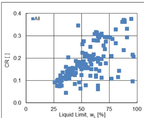
Fig. 10 Plot of Compression Ratio with Liquid Limit: All Sites
