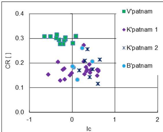
Fig. 9 Plot of Compression Ratio with Consistency Index: Marine Sites
