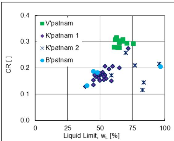
Fig. 5 Plot of Compression Ratio with Liquid Limit: Marine Sites
