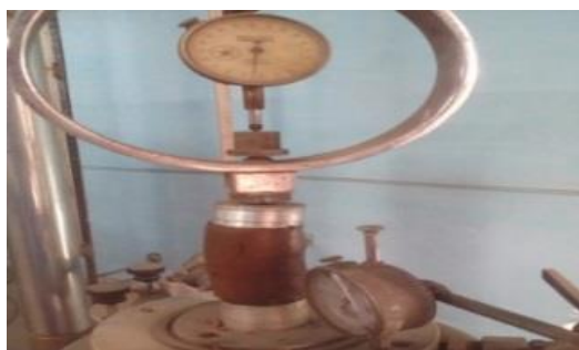
Fig10 Sample during testing on load testing machine
