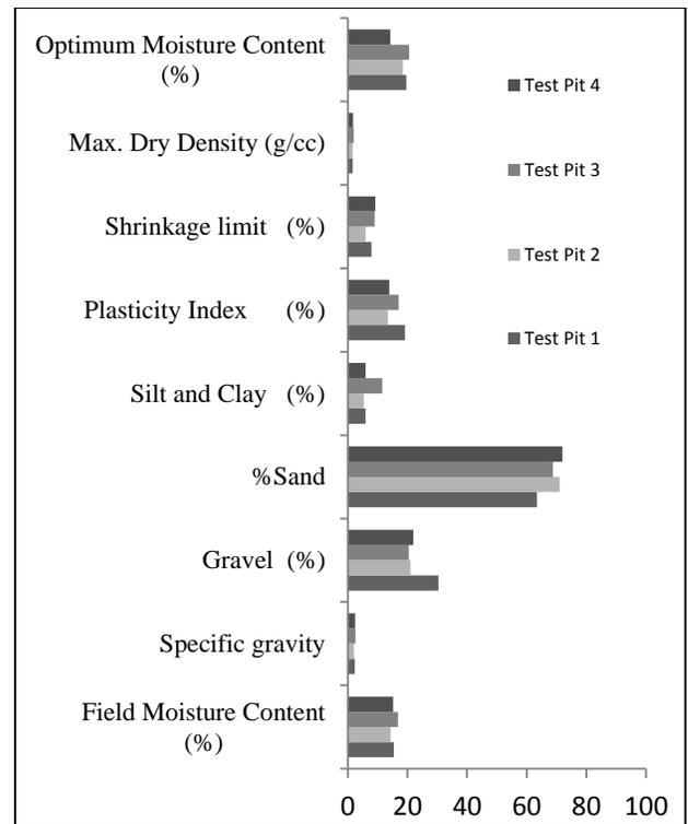
Fig 2: Variation of soil properties in test pits
