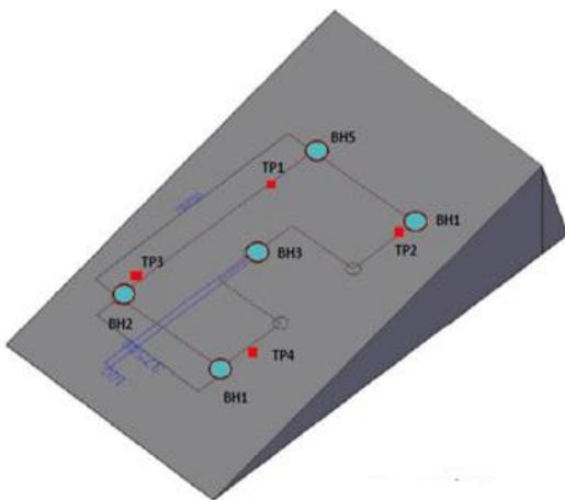
**Fig 3: Location of Test Pits and Bore holes**
