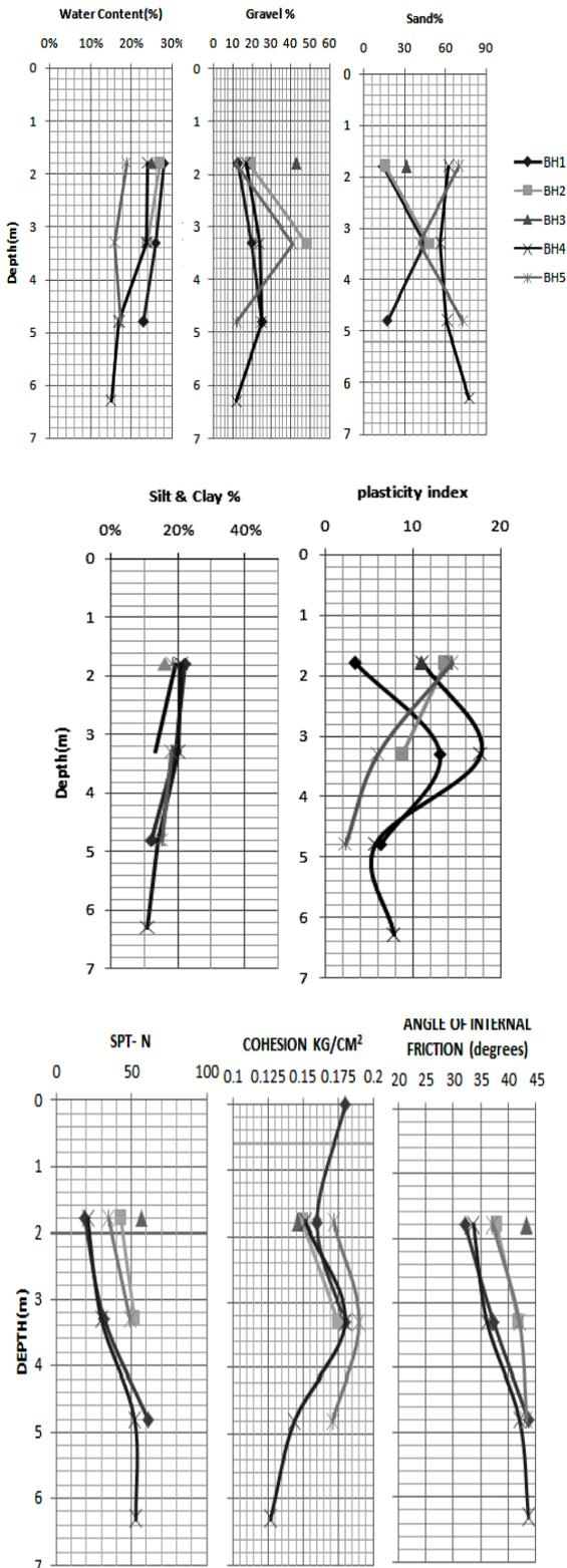
Fig.4: Variability of soil properties with depth
