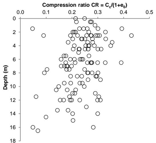
Fig.6 Compression ratio with Depth
