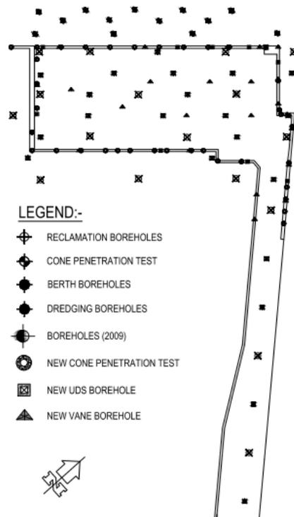
Fig. 1 Geotechnical investigation plan
