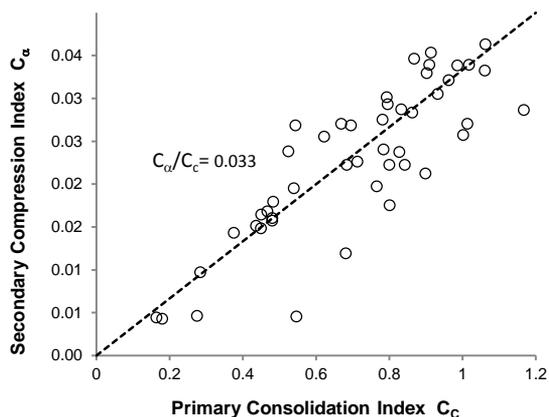
Fig.8 Compression index ratio  $C_{\alpha}/C_c$
