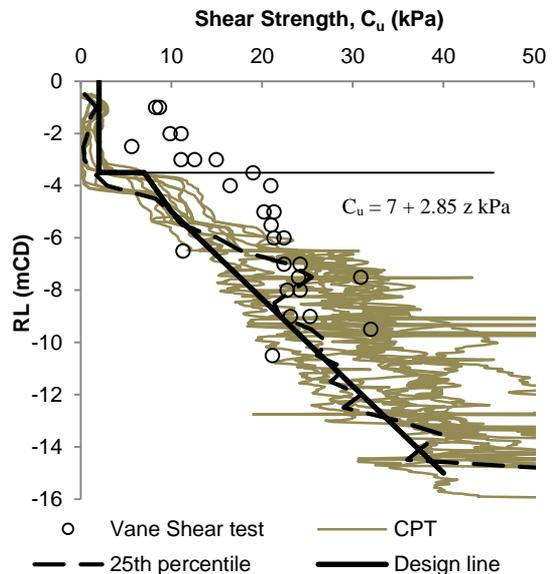
Fig.4 Undrained shear strength with depth
