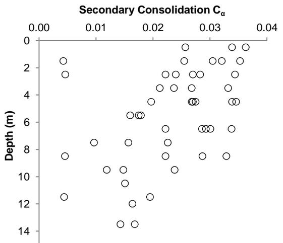
Fig.7 Secondary compression index  $C_\alpha$
