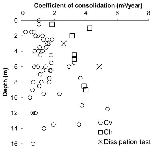
Fig.5 Coefficient of consolidation  $C_v$  &  $C_h$
