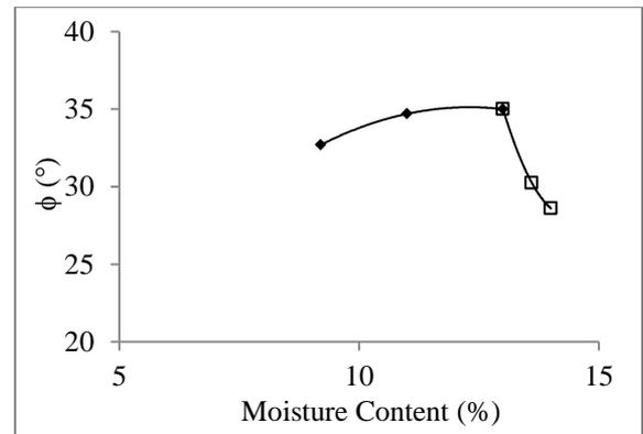
Fig. 4 Variation of  $\phi$  with Moisture Content for soils 2
