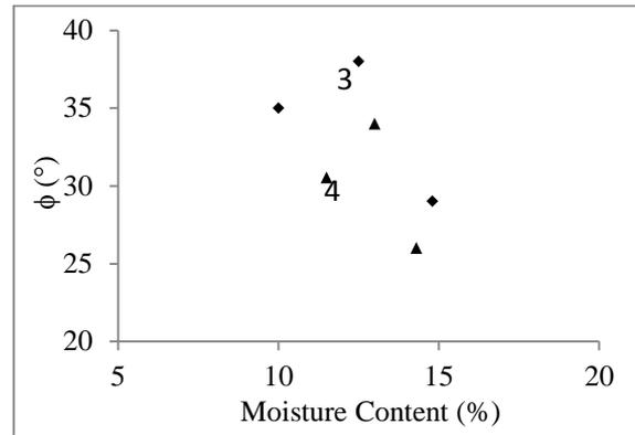
Fig. 5 Variation of  $\phi$  with Moisture Content for soils 3 and 4
