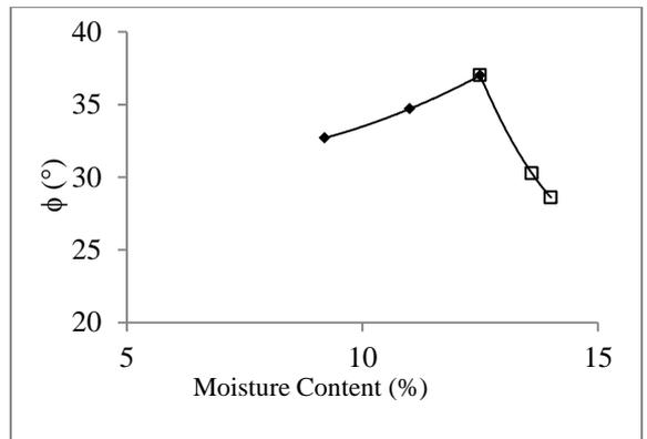
Fig. 3 Variation of  $\phi$  with Moisture Content for soils 1
