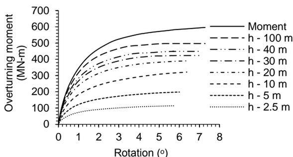
Fig. 2(c) Overturning moment-rotation of bucket foundation (D = 10 m, L = 12 m & V = 30 MN)
