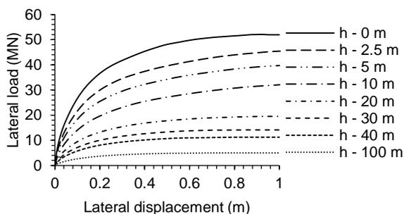
Fig. 2(a) Lateral load-displacement response of bucket foundation (D = 10 m, L = 12 m & V = 30 MN)
