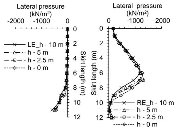
Fig. 7 Lateral pressure along bucket depth
