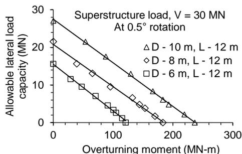
Fig. 8 Interaction diagram at  $0.5^\circ$  rotation
