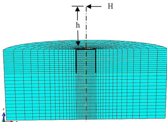
Fig. 1 Discretized bucket foundation soil system
