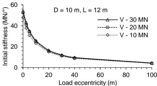
Fig. 4 Initial stiffness of bucket foundation
