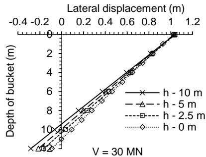
Fig. 6 Depth of point of rotation of bucket foundation (D = 10 m, L = 12 m)
