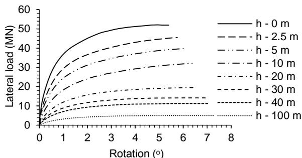
Fig. 2(b) Lateral load-rotation response of bucket foundation (D = 10 m, L = 12 m & V = 30 MN)
