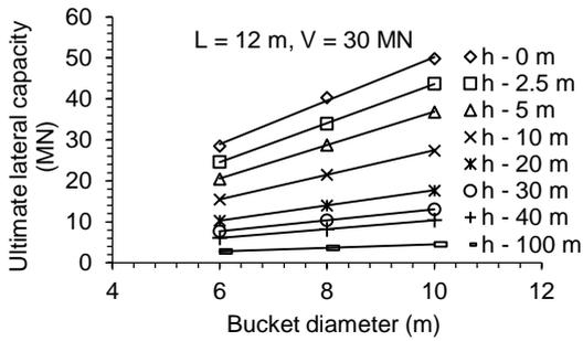
Fig. 3 Ultimate lateral load capacity of bucket foundation
