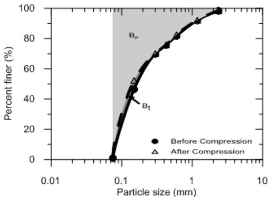
Fig. 3 Grain size distribution of sand B, before and after crushing
