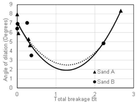
Fig. 5 Variation of Dilatancy angle with Total breakage
