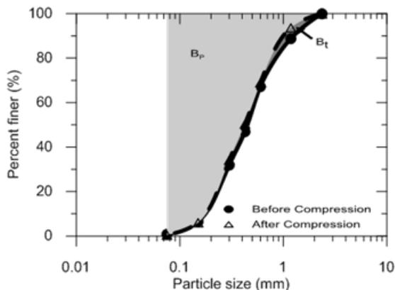
Fig. 1 Grain size distribution curves of sand A, before and after crushing
