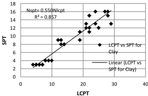
Fig. 3 LCPT resistance vs SPT-N value for clay
