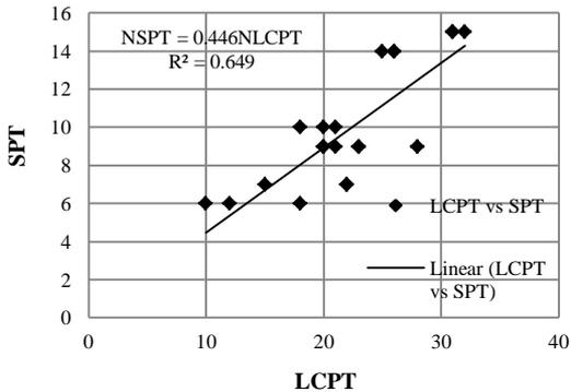
Fig. 2 LCPT resistance vs SPT-N value for sand
