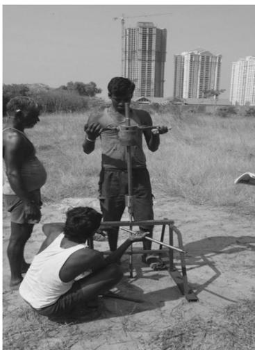
Fig 1 Light cone penetrometer
