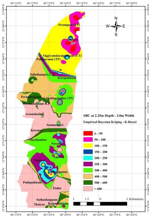
Fig. 6 SBC Map ( $\text{kN/m}^2$ ) at 2.25 m Depth for 2 m Wide Footing
