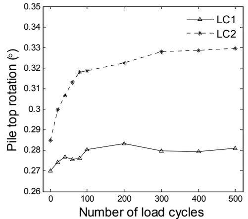
Figure 4. Variation of pile head rotation
