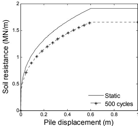
Figure 2.  $p$ - $y$  curves for static and cyclic cases
