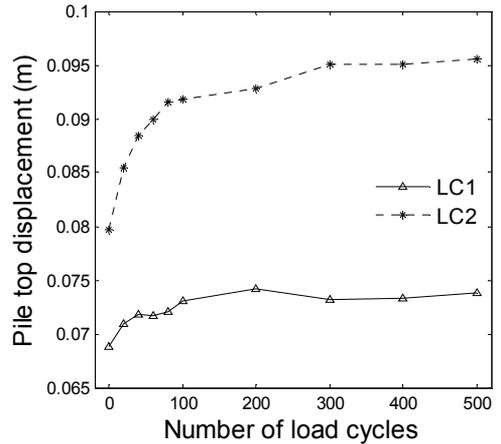
Figure 3. Variation of pile head displacement
