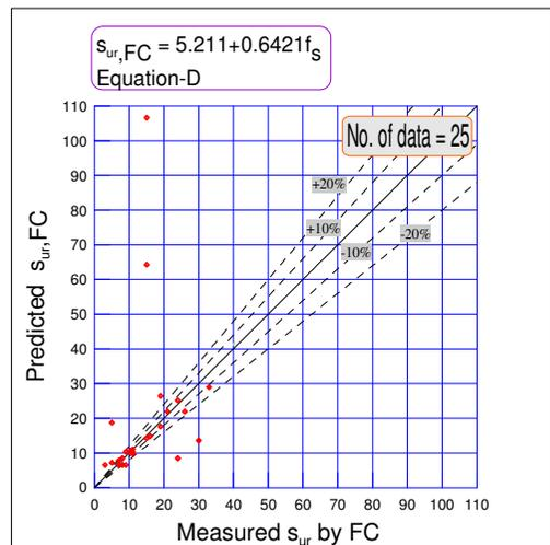
Fig. 5 Predicted Remoulded shear strength from Eqn. D vs. Measured Remoulded shear strength (fall cone)
