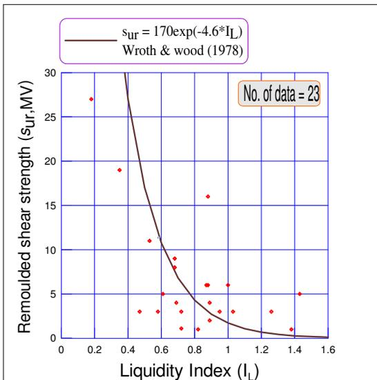
Fig. 1 Evaluation of correlation for Remoulded shear strength by Wroth & wood (1978) for the soil data from western Indian Offshore (Miniature Vane)
