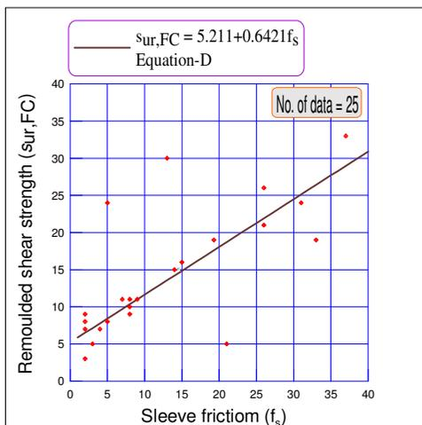
Fig. 4 Evaluation of correlation of remoulded shear strength by regression analysis (Eqn. D) for the soil data from western Indian Offshore (fall cone)
