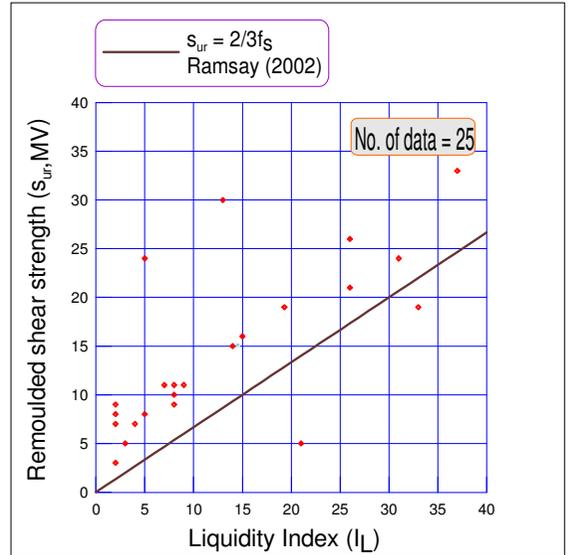
Fig. 2 Evaluation of correlation for Remoulded shear strength by Ramsay (2002) for the soil data from western Indian Offshore (Miniature Vane)
