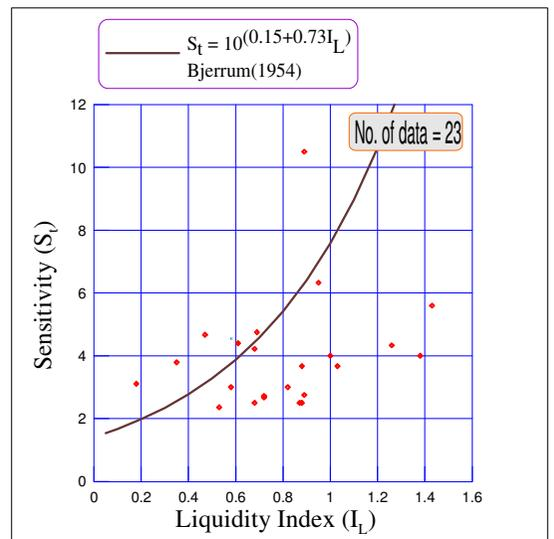
Fig. 3 Evaluation of correlation for sensitivity by Bjerrum (1954) for the soil data from western Indian Offshore (Miniature Vane)
