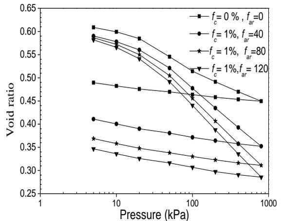
**Fig. 3** Void ratio vs. Pressure
