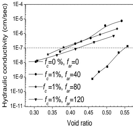
Fig.5 Void ratio- hydraulic conductivity at fixed  $f_c=1\%$
