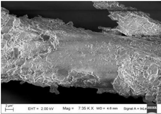
Fig.4 Roughness of glass fiber after test
