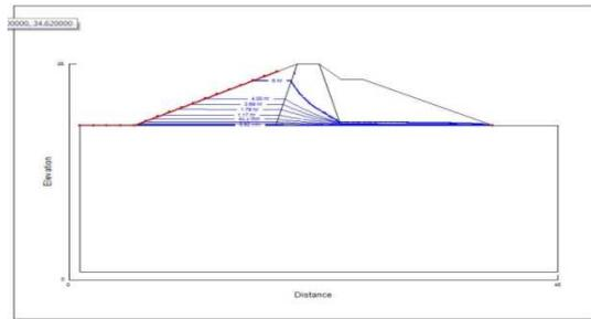
Fig. 5 Iso-line of Phreatic Surface of Earthen dam with clay core for draw down rate= 0.85 m /hour for (t)= 0 sec to 21600 sec.
