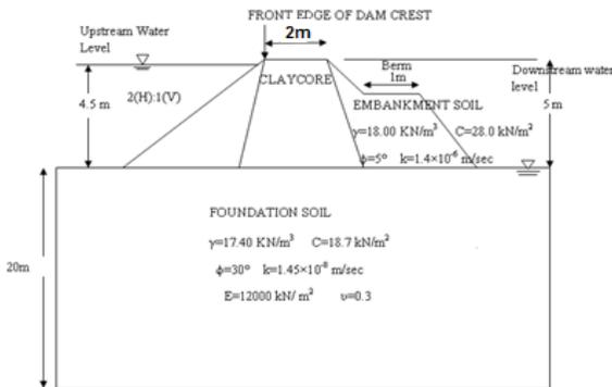
Fig. 1: Schematic diagram of dam with details
