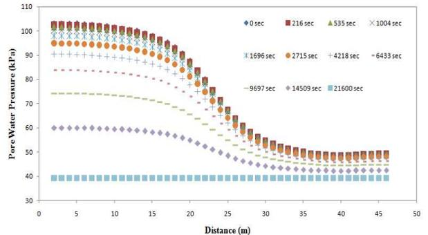
Fig. 8 Pore water pressure variation of earthen dam with clay core for drawdown rate= 0.85 m /hour for time (t) = 0 Sec to 21600 Sec (5m below the embankment)
