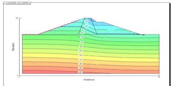
Fig. 7 Earthen dam with clay core for drawdown rate= 0.85 m /hour for time (t) =9697 Sec
