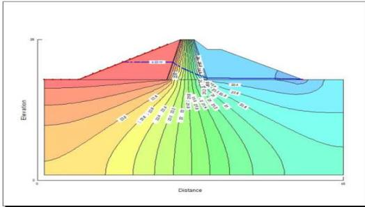
Fig. 3 Earthen dam flow net with clay core for draw rate = 0.85 m /hour and t= 9697Sec
