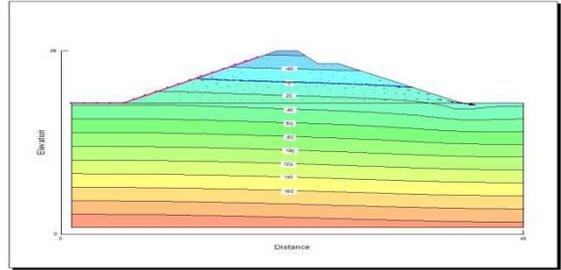
Fig. 6 Pore water pressure variation of Earthen dam with out clay core for drawdown rate= 0.85 m /hour for time (t) =9697 Sec
