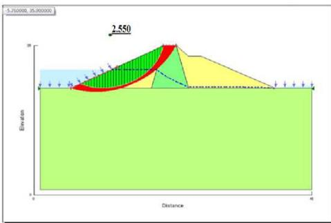
Fig. 9 Factor of safety of earthen dam with clay core for drawdown rate= 0.85 m /hour for time (t) = 14509 sec during a Single Tidal Cycle
