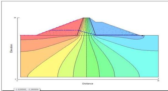
Fig. 4 Earthen dam flow net with clay core for draw rate = 0.85 m /hour and t= 9697Sec
