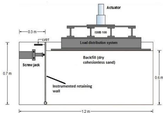
Fig. 1 Detailed experimental setup used in model tests
