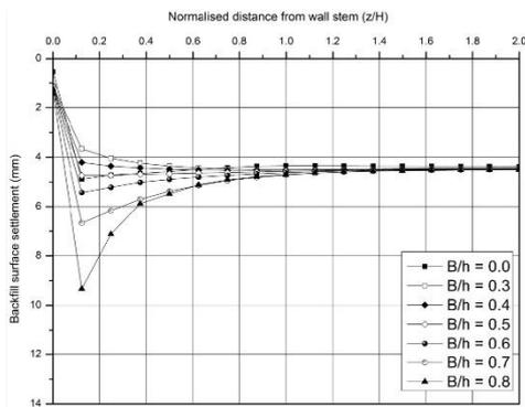
Fig. 7 Backfill Surface settlement profile of backfill
