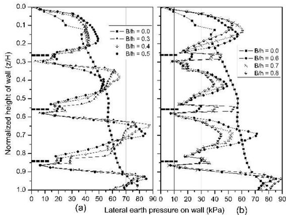
Fig. 4 (a) and (b) Comparison of lateral earth pressure on the wall with and without relief shelves
