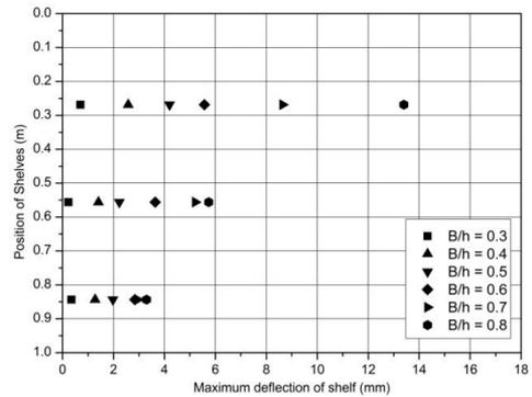
Fig. 6 Maximum vertical deflection (mm) profile of relief shelves
