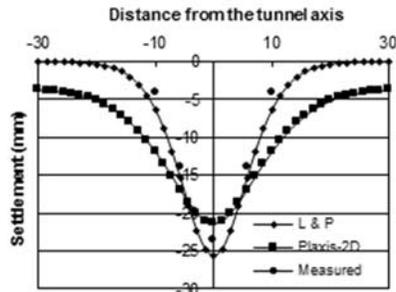
Fig. 1.0 Predicted and observed settlement trough.
