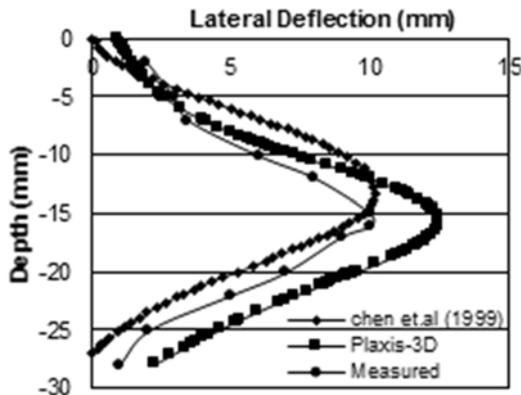
Fig. 3.0 Measured and predicted pile lateral deflection
