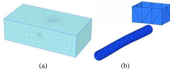
Fig. 4: Typical FE mesh (a) meshed ground (b) meshed lining and raft-retaining wall
