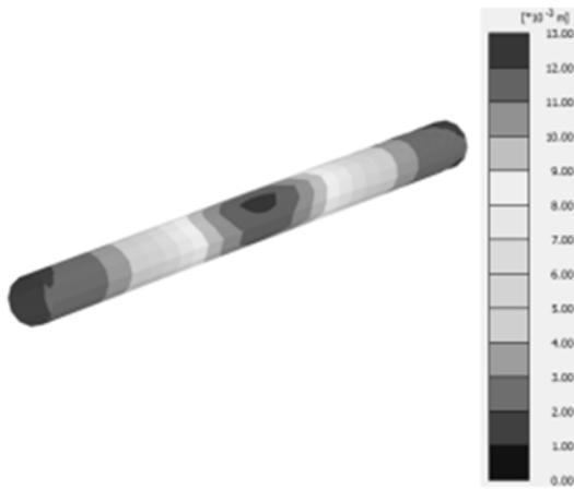
Fig. 5: Predicted displacement contour of complete FE mesh
