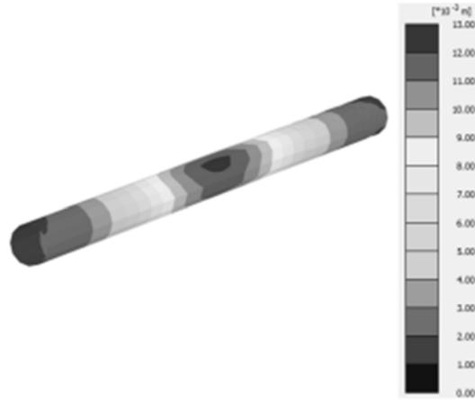
Fig. 6: Predicted displacement contour of tunnel lining.
