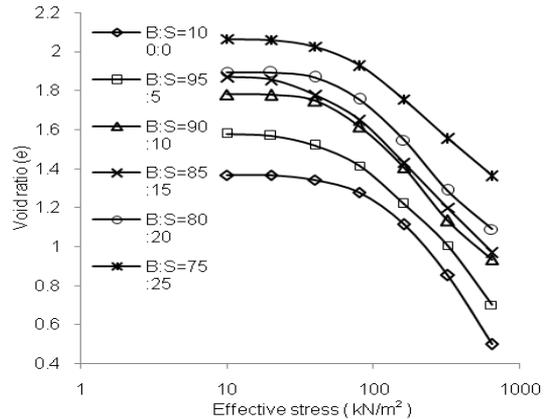
Fig. 5 Relationship between void ratio and effective stress ( $\sigma'_v$ ) plot for the six samples.
