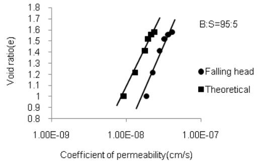
Fig.8b Comparison of permeability calculated experimentally and theoretically for B:S=95:5
