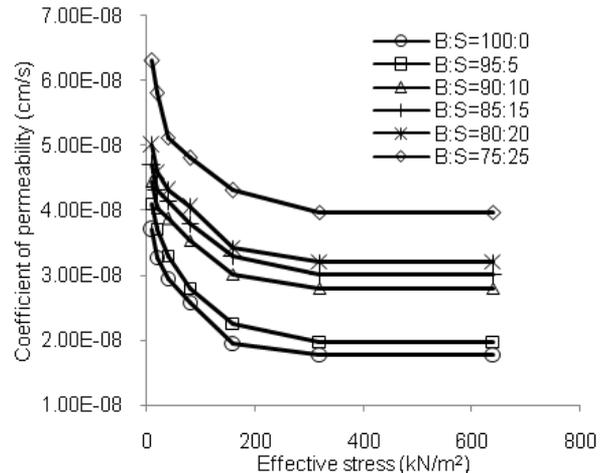
Fig. 6 Relationship between effective vertical stress and coefficient of permeability calculated experimentally.
