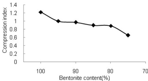
Fig. 4 Compression index versus bentonite content
