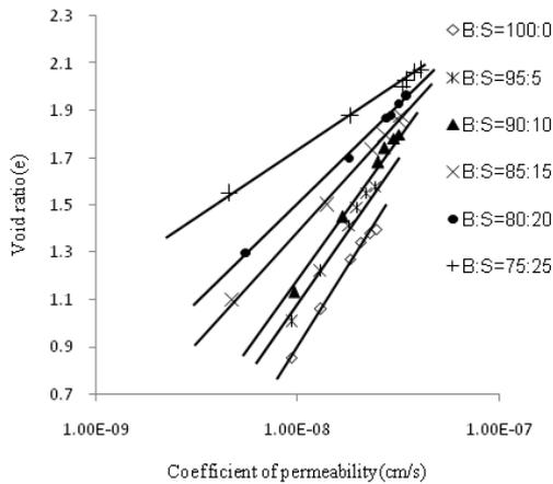
Fig. 7 Void ratio Vs coefficient of permeability ( $k$ )
