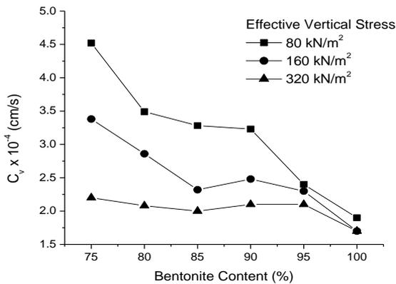
Fig. 3 Coefficient of consolidation versus bentonite content
