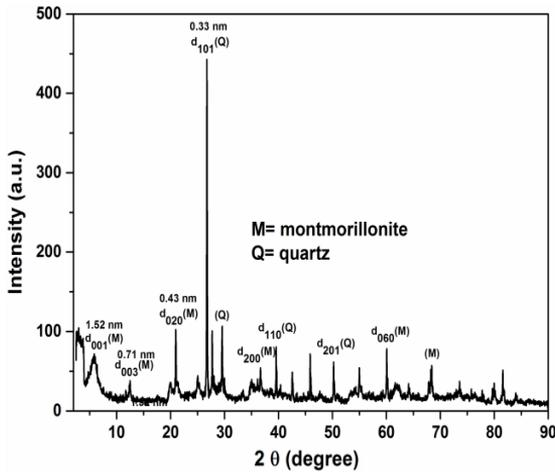
Fig. 1 The X-ray diffraction pattern for the bentonite
