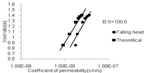
Fig.8a Comparison of permeability calculated experimentally and theoretically for pure bentonite
