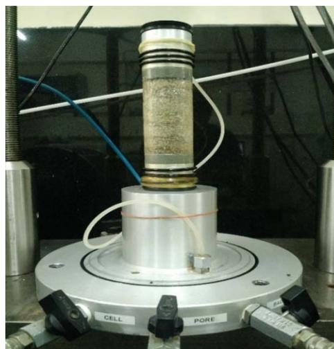
Fig. 4 Specimen prepared from sand-rubber tyre shreds mixture
