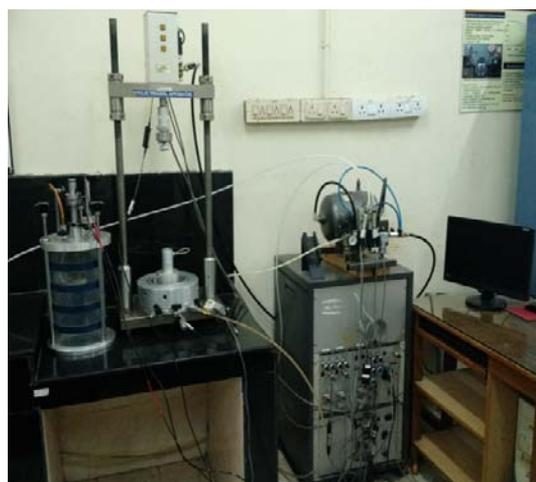
Fig. 3 Cyclic Triaxial Apparatus
