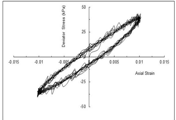
Fig. 5 Typical hysteresis loops for 50% rubber content showing 25 number of cycles at 1% strain
