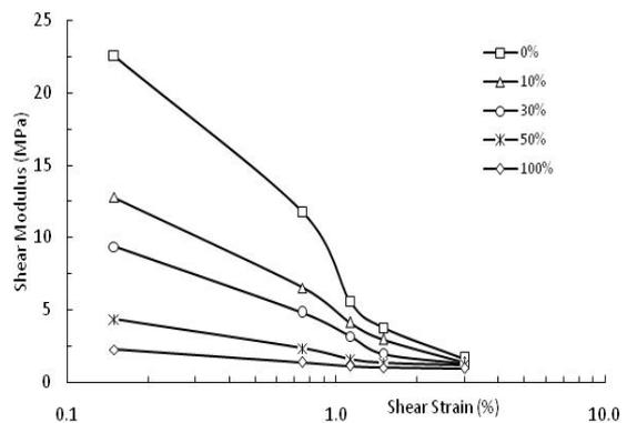
Fig. 7 Plot of shear modulus versus shear strain for sand-rubber tyre shreds mixtures
