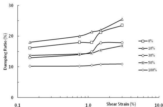
Fig. 8 Plot of damping ratio versus shear strain for sand-rubber tyre shreds mixtures
