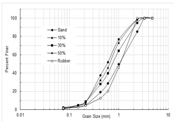
Fig.1 Particle size distribution curves for sand-rubber tyre shreds mixtures
