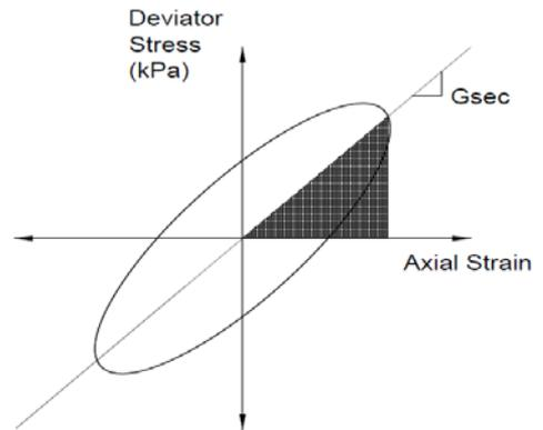
Fig. 6 Schematic diagram of hysteresis loop
