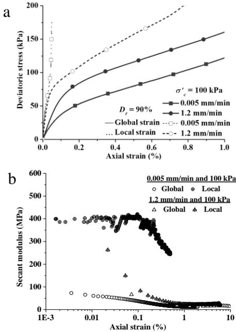
Fig. 6 Variation of (a) global and local stress-strain and (b) soil stiffness at two different displacement rates
