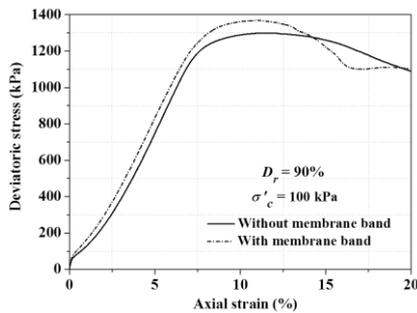
Fig. 7 Response of soil on the use of rubber strip
