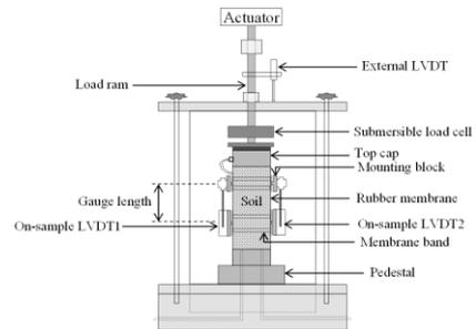
Fig. 4 Schematic diagram of the use of on-sample LVDTs
