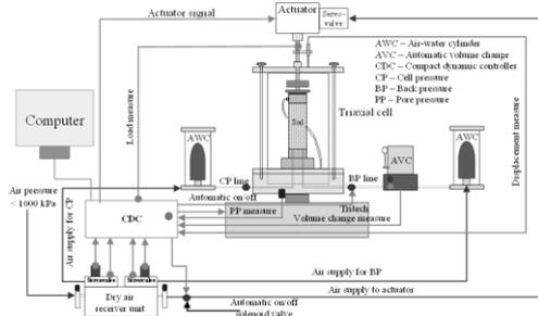
Fig. 3 Layout of cyclic triaxial test setup
