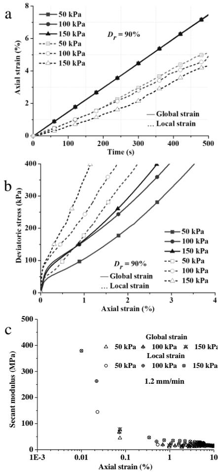
Fig. 5 Variation of (a) global and local strain (b) Stress-strain response and (c) soil stiffness with on-sample and external LVDTs
