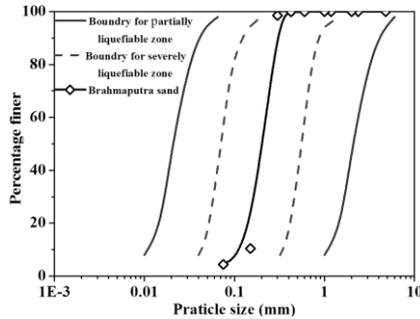
Fig. 2 Particle size distribution
