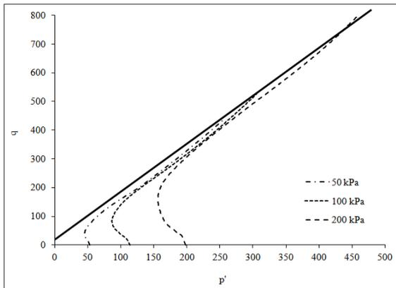
Figure 4:  $p'$ - $q$  plot of Consolidated Undrained triaxial test of IITG Cut Slope Site sample
