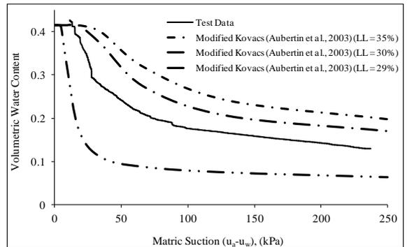
Figure 5: Soil Water Characteristic Curves for the saprolitic soil (PGSS\_EXP2)
