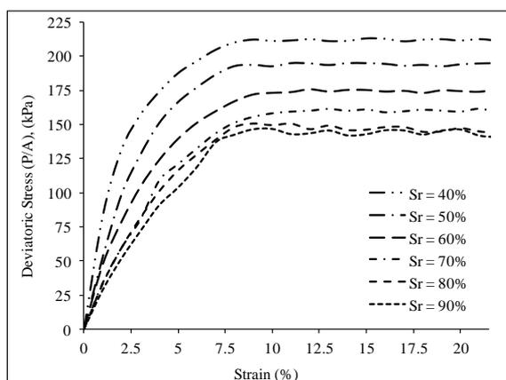
Figure 6: Deviatoric Stress vs. Strain (%) for partially saturated soil sample.
