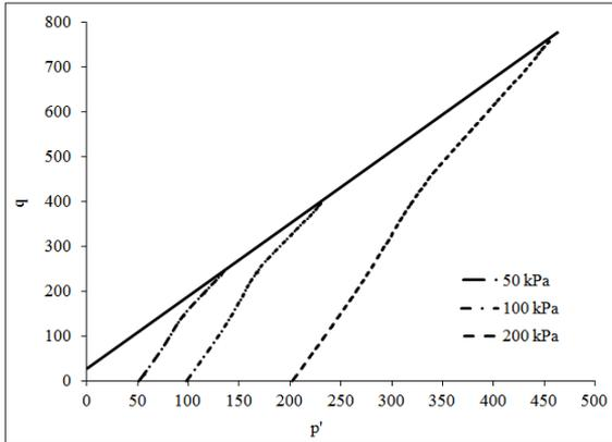
Figure 3:  $p'$ - $q$  plot of Consolidated Drained triaxial test of IITG Cut Slope Site sample
