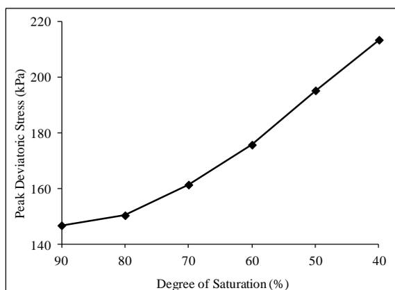
Figure 7: Increase in Peak Deviatoric Stress with decrease in Degree of Saturation (%)
