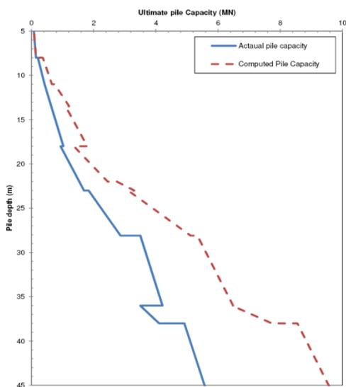
Fig. 2 Comparison of predicted and actual pile axial capacity
