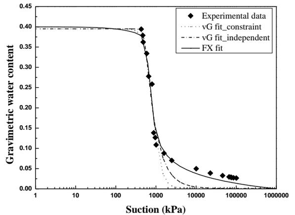
Fig. 5 Comparison of FX and vG fit for S2
