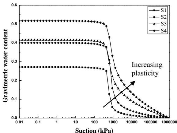
Fig. 8 Comparison of FX model fit for the four soils
