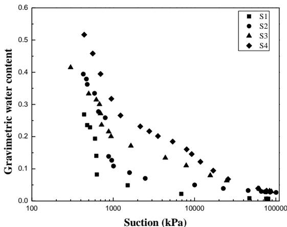
Fig. 3 Measured SWCC of the used soils
