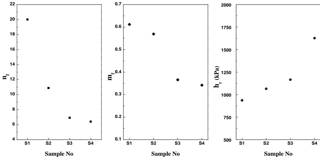
Fig. 9 Comparison of different FX model parameters of the used sample
