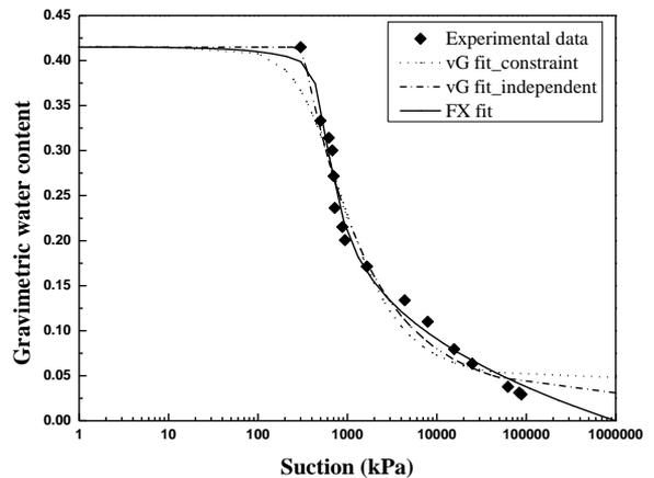
Fig. 6 Comparison of FX and vG fit for S3
