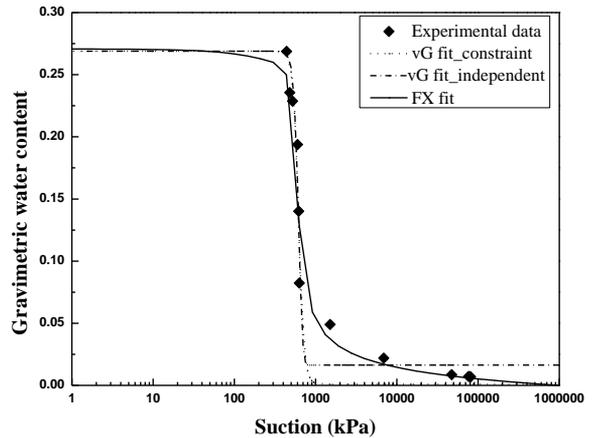
Fig. 4 Comparison of FX and vG fit for S1
