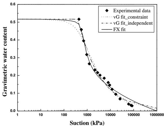
Fig. 7 Comparison of FX and vG fit for S4
