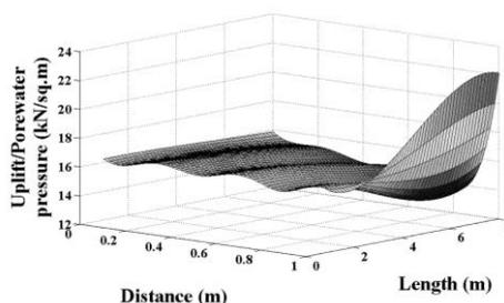
Fig. 3 Variation of uplift and toe pore-water pressure
