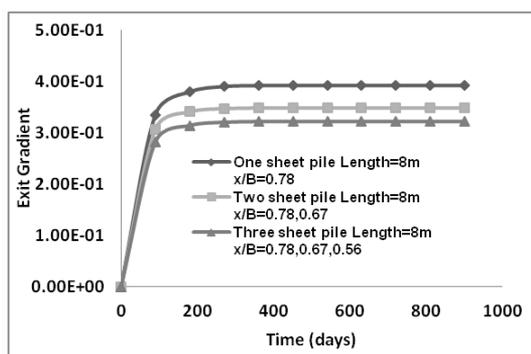
Fig.5 Variation of exit gradient with time
