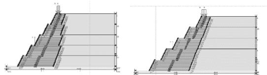
**Fig 1.** Typical geometry model (a) 30m height with 1.5m berm width (b) 30m height with 3.0m berm width
