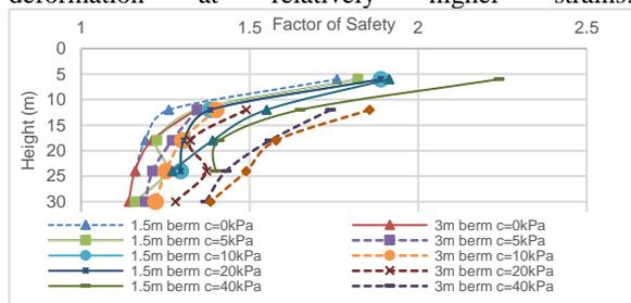
Fig. 5 Graph depicting trend of factor of safety w.r.t height of slope embankment.
