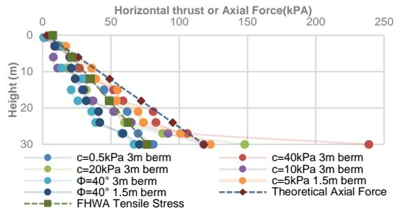
**Fig.2** Graphical Representation of observe trend of acting axial forces over geogrids with respect to height (30m)
