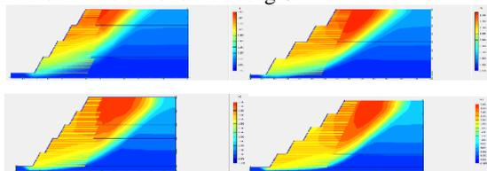
Fig.6. Typical graphical plot of total maximum displacements (shear surface or slip circles) (a) 24m 1.5m berm, (b) 24m 3.0m berm, (c) 30m 1.5m berm, (d) 30m with 3.0m berm
