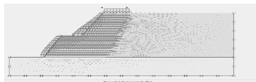
**Fig.4** Screenshot: Typical Observed Trend for Maximum horizontal displacement (After staged construction analysis)
