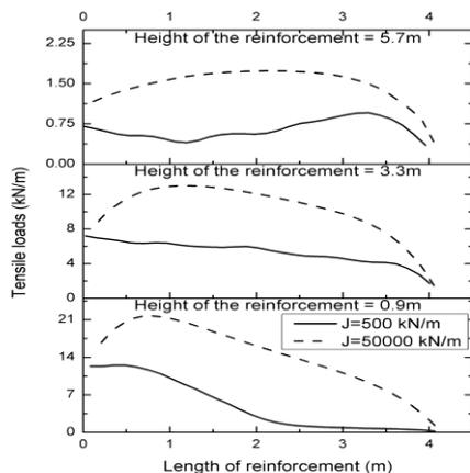
Fig. 5 Tensile force profile along the reinforcement length at different heights for unconnected case ( $W/H=2.0$ )
