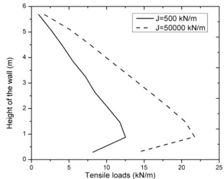
Fig. 6 Maximum tensile forces profile for unconnected case ( $W/H=2.0$ )
