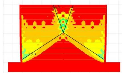
Fig. 3 Maximum shear strain increment contour for the case  $J=500$  kN/m and  $W/H=1.40$  unconnected reinforcement
