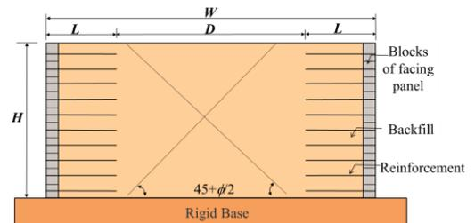
Fig. 1 Schematic of back-to-back MSE walls
