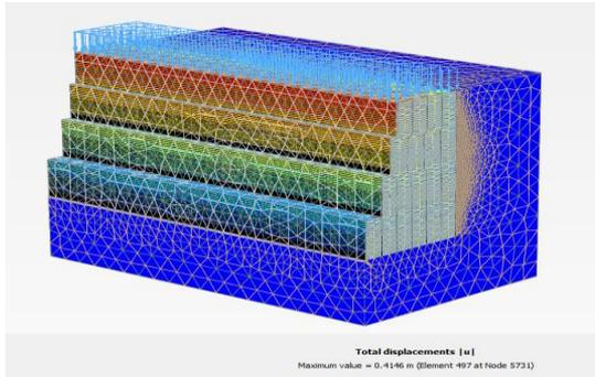
**Fig 3** Failure pattern of wall for Hardening soil model
