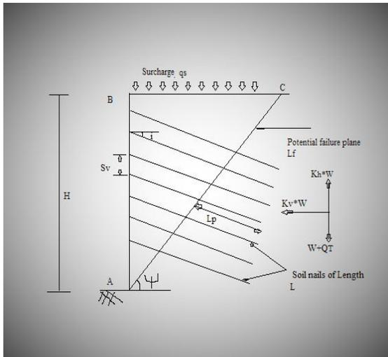
Figure 5. Forces acting on soil nail wall under dynamic condition
