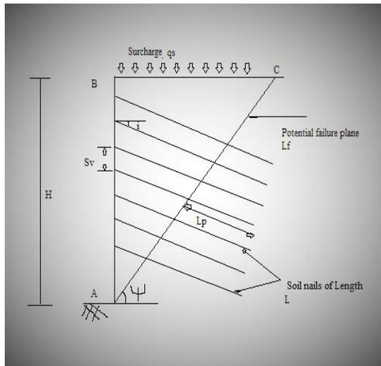
Figure 1. Typical soil nail wall design parameters
