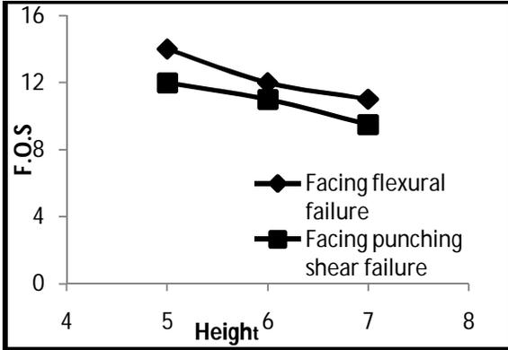
Figure 4: Height v/s F.O.S for facing flexural and facing punching shear failure
