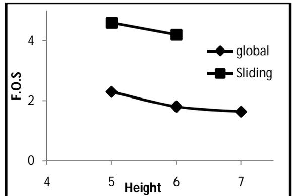
Figure 2: Height v/s F.O.S for global and sliding stability
