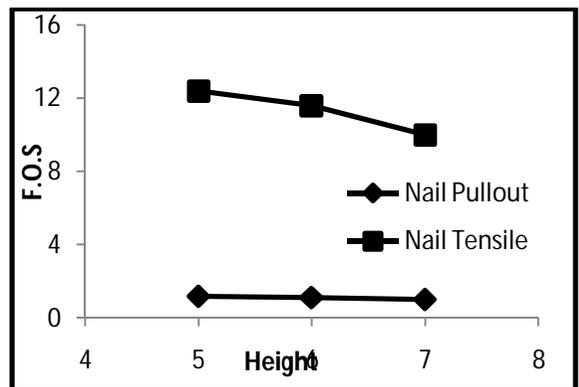
Figure 3: Height v/s F.O.S for nail pullout and nail tensile failure
