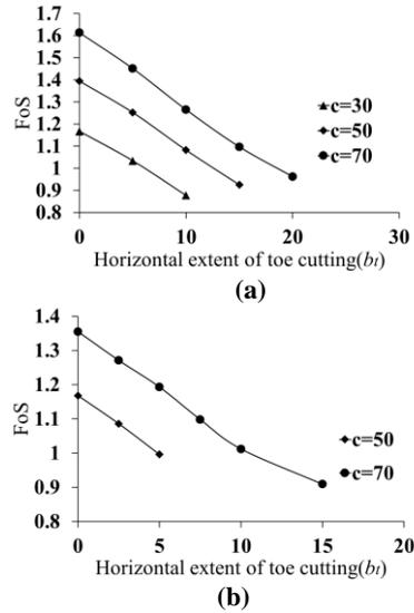
Fig. 4 Effect of toe cutting on dry hill slopes for (a)  $\beta=50^\circ$ ,  $\varphi=35^\circ$  (b)  $\beta=60^\circ$ ,  $\varphi=35^\circ$
