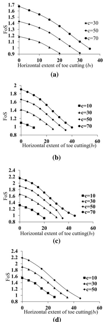
Fig. 2 Effect of toe cutting on dry hill slopes for  $\beta=30^\circ$ , (a)  $\phi=20^\circ$  (b)  $\phi=25^\circ$  (c)  $\phi=30^\circ$  (d)  $\phi=35^\circ$
