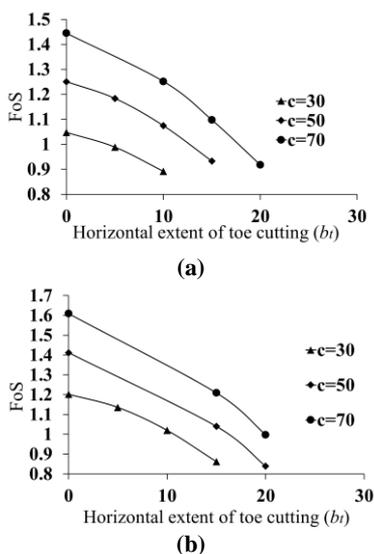
Fig. 6 Effect of toe cutting on partially saturated slopes for (a)  $\beta=40^\circ$ ,  $\phi=30^\circ$  (b)  $\beta=40^\circ$ ,  $\phi=35^\circ$
