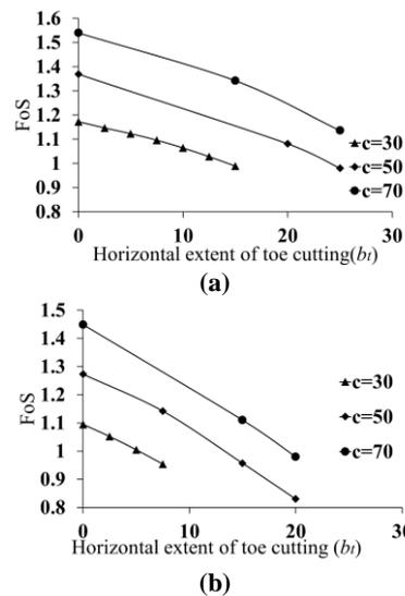
Fig. 5 Effect of toe cutting on dry hill slopes with pseudo-static earthquake for (a)  $\beta=30^\circ$ ,  $\varphi=30^\circ$  (b)  $\beta=40^\circ$ ,  $\varphi=35^\circ$
