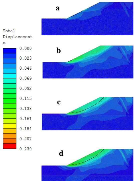
Fig.5 Contours of total displacements from FEM and critical surface from LEM for case-2 and layer height (a)  $h=0.2D$  (b)  $h=0.4D$  (c)  $h=0.6D$  and (d)  $h=0.8D$
