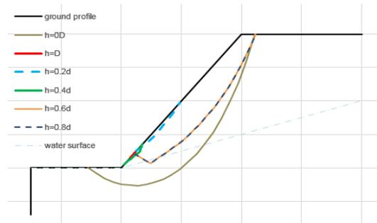
Fig.4 Critical surfaces for various layer heights for case-2 using the limit equilibrium method
