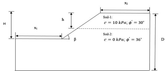
Fig.2 Non-homogeneous slope model
