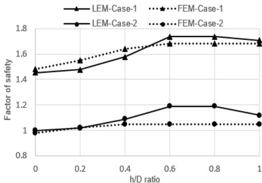
Fig.6 Variation of safety factor with height ratio for case-1 and 2
