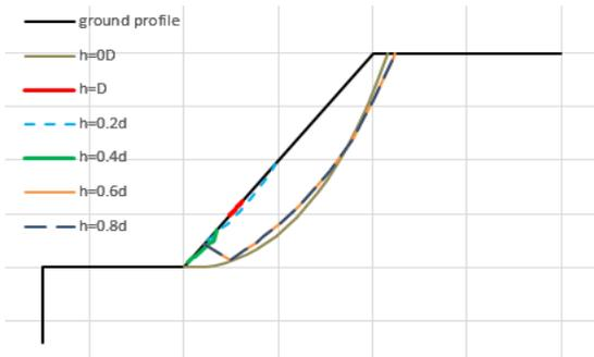
Fig.3 Critical surfaces for various layer heights for case-1 using the limit equilibrium method
