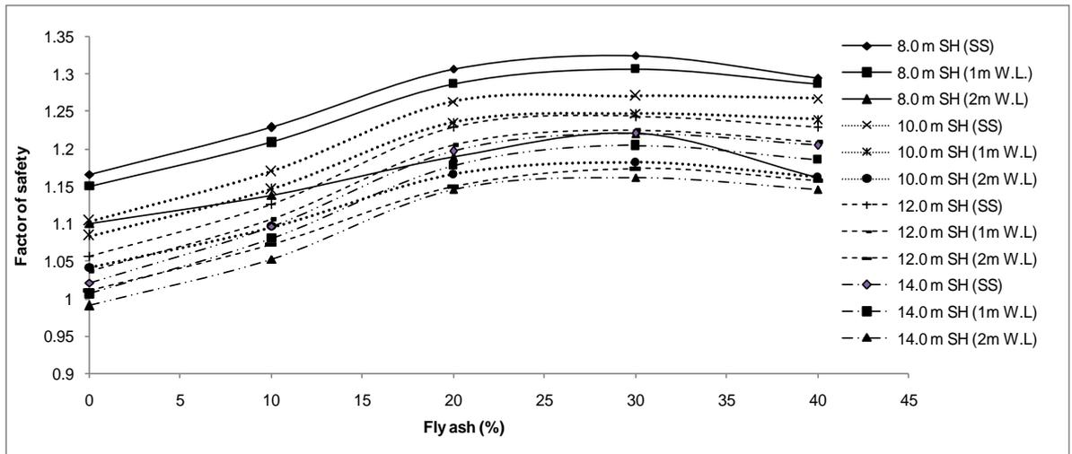
Fig. 6 Variation in FoS with different slope height and fly ash content at summer and rainy season.
