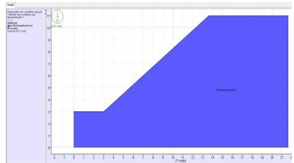
Fig. 2 Geometric model of embankment slope with native soil during summer season.
