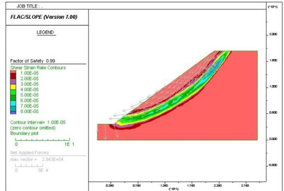
Fig. 4 Shear strain rate contour for native soil slope of 14.0 m height and 2.0 m water level (FoS=0.99).
