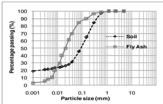
Fig. 1 Particle size distribution curve of soil and fly ash.
