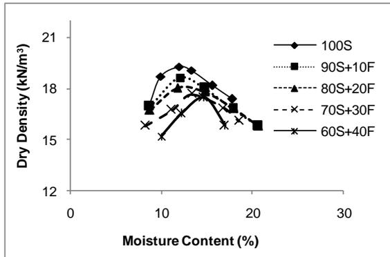
Fig. 3 Compaction Curve for all samples.
