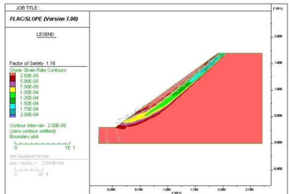
Fig. 5 Shear strain rate contour for stabilized soil with 30% fly ash slope of 14.0 m height and 2.0 m water level (FoS=1.162).
