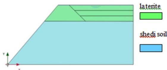
Fig. 2 Geometric profile of the slope
