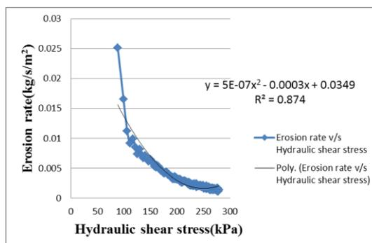
Fig. 1 Erosion rate v/s hydraulic shear stress for F1 sample
