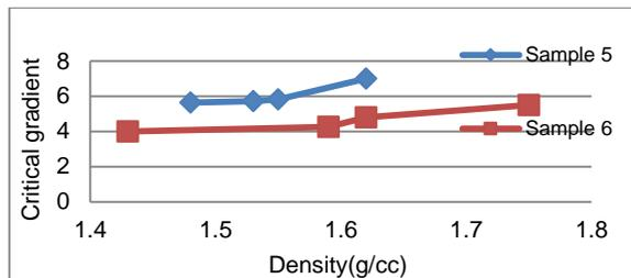
Fig. 7 – Density Vs Critical Hydraulic gradient
