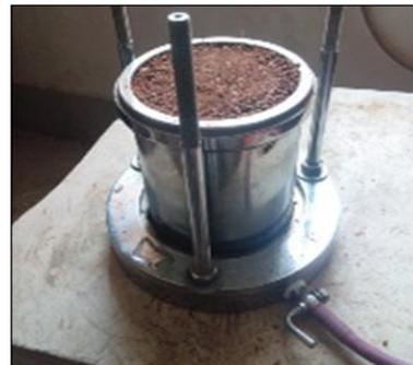
Fig 2- Cylindrical mould compacted with soil
