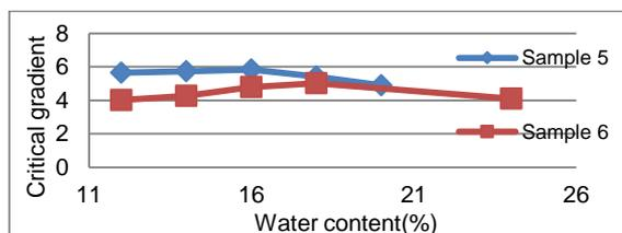
Fig 8 – Water content Vs Critical Hydraulic gradient
