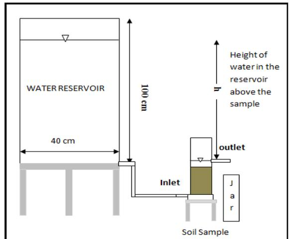
Fig 1- Experimental Setup (Not drawn to scale)
