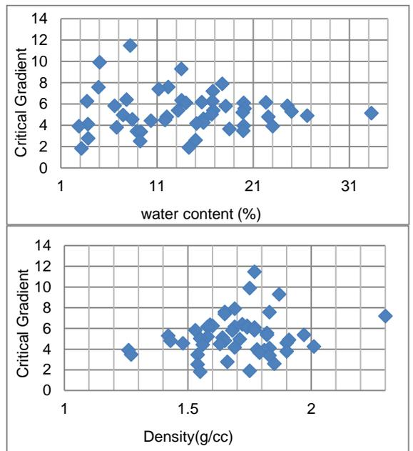
Fig 6 -Variation of Critical Hydraulic Gradient with Density and Water content
