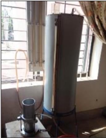
Fig 3- Mould connected to the water reservoir
