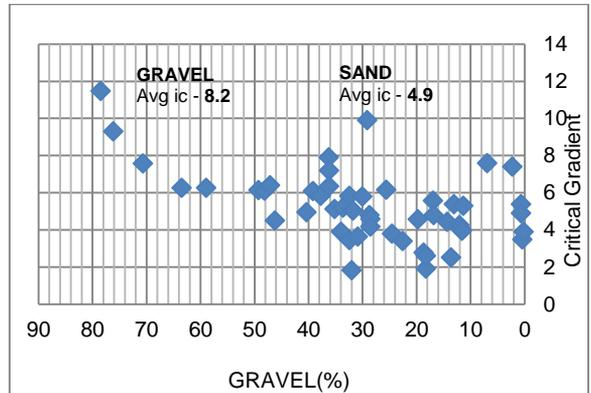
Fig 5 – % Gravel Vs Critical Hydraulic Gradient
