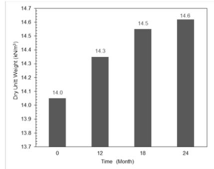
Fig. 4 Dry unit weight versus time curve for field JGT reinforced rural road section.
