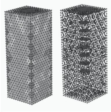
Fig. 2 Plaxis model of Granular piles reinforced with 50 mm spaced horizontal strips
