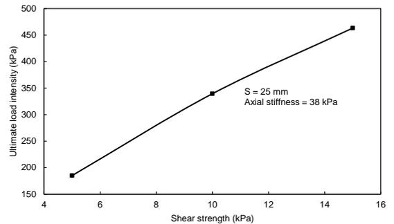
Fig. 4 Variation of the ultimate load intensity with undrained shear strength of clay
