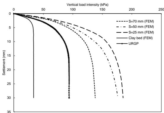
Fig. 3 Vertical load intensity settlement behaviour of horizontal reinforced floating granular piles
