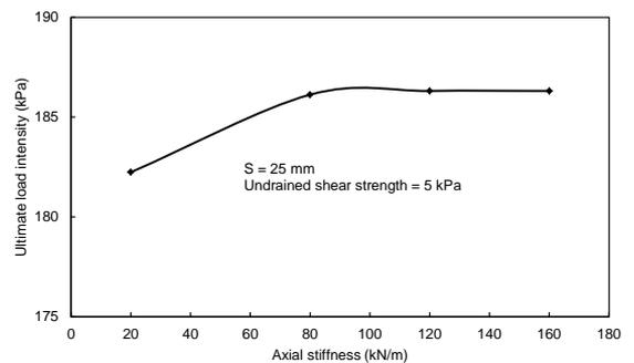
Fig. 5 Variation of the ultimate load intensity with axial stiffness of geogrid
