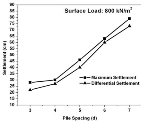
Fig. 5 Differential settlement with varying pile spacing
