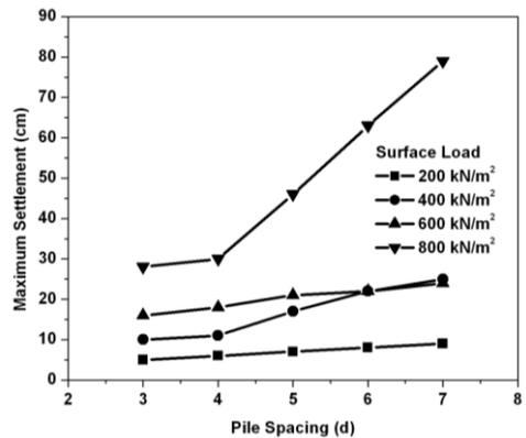
Fig. 4 Maximum settlement with varying pile spacing
