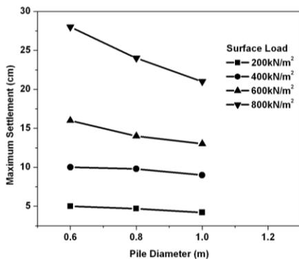
Fig. 6 Maximum settlement with varying pile diameter
