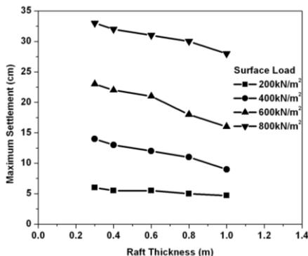
Fig. 2 Maximum settlement with varying raft thickness
