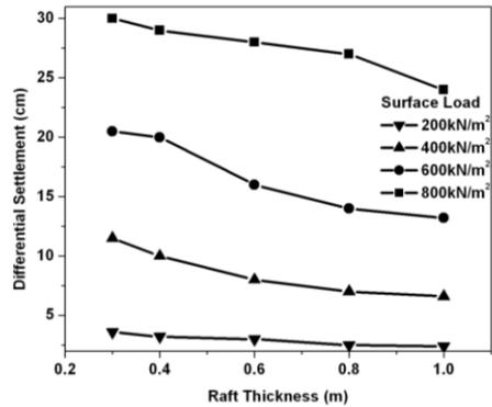
Fig. 3 Differential settlement with varying raft thickness
