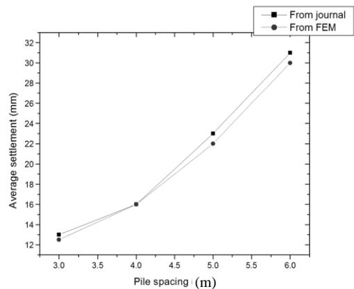
Fig. 1 Average settlement vs. pile spacing
