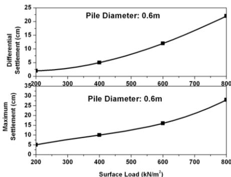
Fig. 7 Non-linear variation of settlement with load
