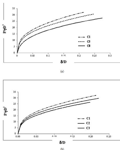
Fig. 5 Normalized load-displacement curve for isolated helical anchor with a) same depth of lower-most helical plate, b) three helical plates
