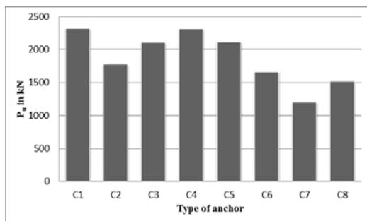
Fig. 7 Variation of  $P_u$  for different anchor configurations
