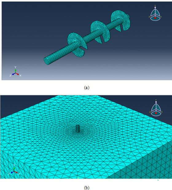
Fig. 3 Overview of a) AutoCAD drawing and finite element meshing of C1 anchor, b) finite element meshing of soil domain
