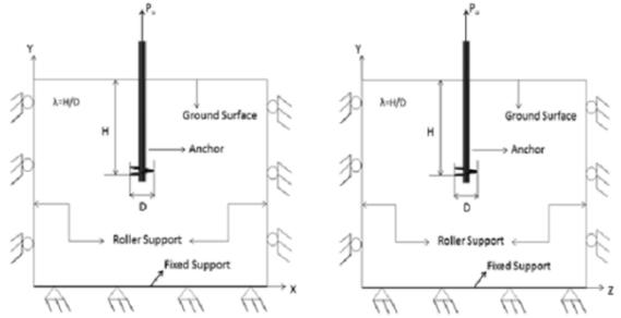
Fig. 4 Boundary conditions along XY and YZ plane
