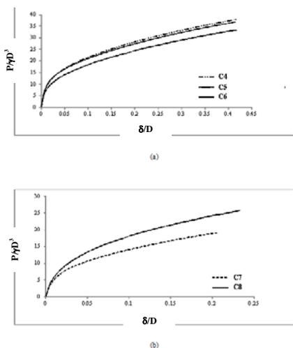
Fig. 6 Normalized load-displacement curve for isolated helical anchor with a) two helical plates, b) single helical plate
