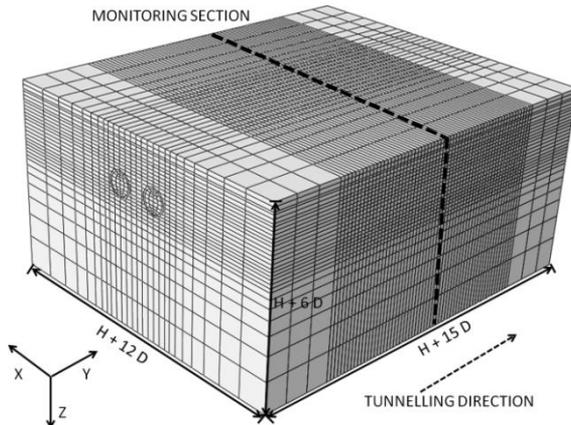
Fig.2 The 3 D finite element mesh for the underground tunnel model considered in this study
