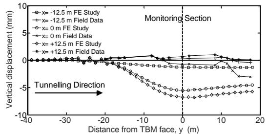
Fig. 3 Vertical displacement at selected locations during the tunnel advancement plotted against the distance of the TBM face from the monitoring section.
