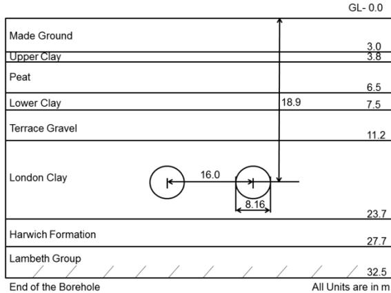
Fig.1 Cross- section of the twin- tunnel alignment
