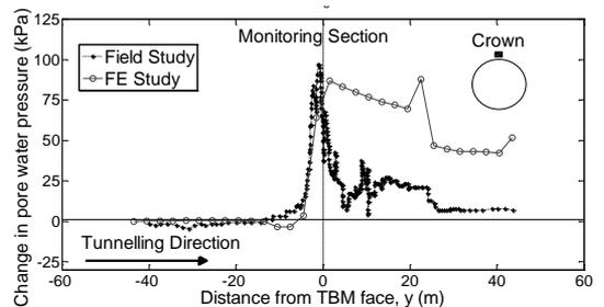
Fig. 4 Pore water pressure variation near the tunnel crown during the tunnel advancement plotted against the distance of the TBM face from the monitoring section.
