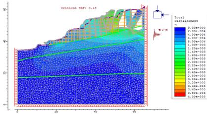
Fig. 5 Max. Deformed shear strain plot of 65 m chainage section with  $K_h = 0.16$
