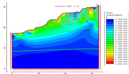
Fig. 4 Total displacement contour plot at critical SRF of section at 65 m chainage
