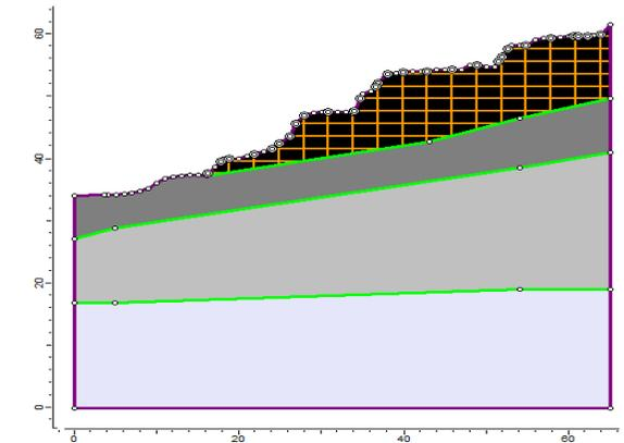
Fig. 3 Geometry and formation of the four rock mass at 65 m chainage.
