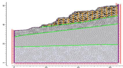
Fig. 3 Discretized phase2 model of slope Section at 65m chainage.
