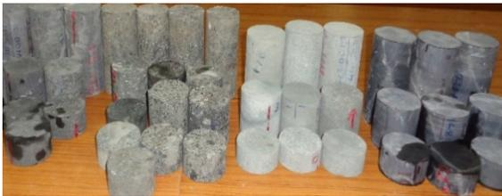
Fig. 2 Specimen prepared for testing under tensile, uniaxial and triaxial loading.
